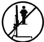
**3.1** - The TE-06 is a machine designed to elevate loads upwards in a vertical direction. It should NEVER be used as a platform to elevate people.
