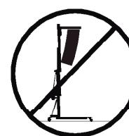
**3.4** - This lift should NEVER be used to elevate a load that has not been properly checked. It is necessary to verify that the load is correctly supported and centred on the appropriate lift support so that the weight of the load will only elevate in a vertical direction.
